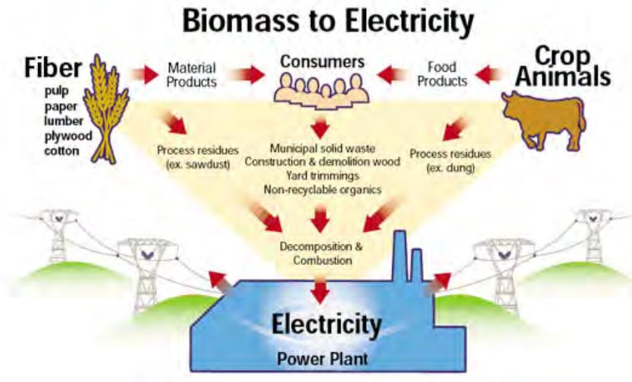
The biomass is then placed into a furnace and burned, or the methane gas in a liquid or gaseous state from algae or rotting / decomposing materials is captured. The heat generated is used to boil water. The steam from the boiling water is used to turn turbines and generators to produce electricity.
