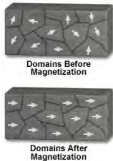
is used to introduce a current through the wire. This creates a magnetic field around the coiled wire, magnetizing the metal as if it were a permanent magnet. It aligns all of the domains in the metal in one orientation. Electromagnets are useful because the magnet can be turned on and off by completing or interrupting the circuit.
